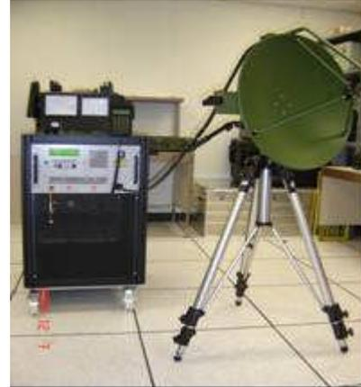
**Preliminary test results.** Laboratory testing has demonstrated very good fidelity on threat reproduction at the TWTA output. Minimum pulse widths of 100 nsec are achievable, with pulse repetition frequencies (PRF's) up to 100 kHz. Measured amplitude modulations agreed with programmed values.
