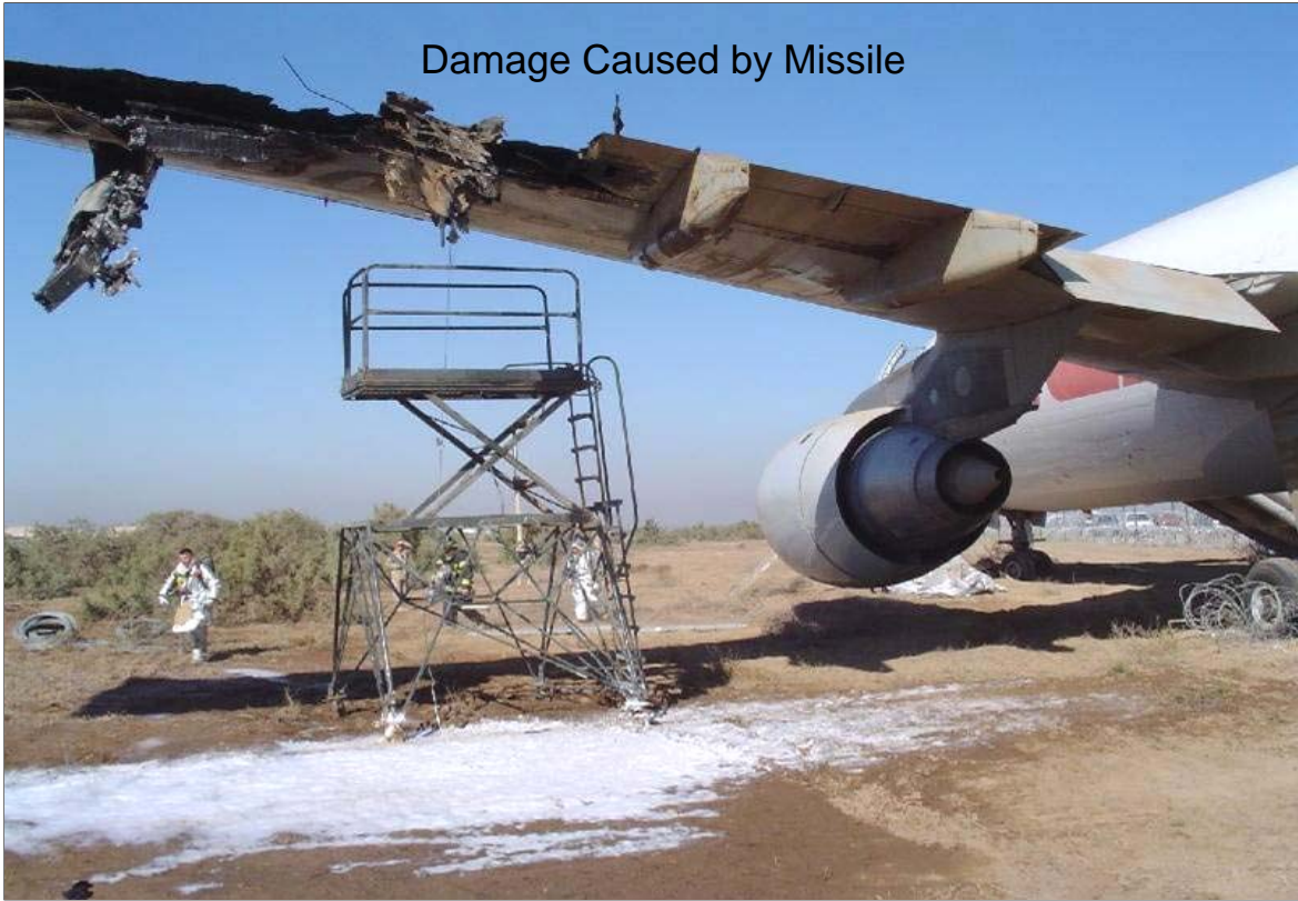
The missile hit the wing, not the engine – that was the lucky part.
