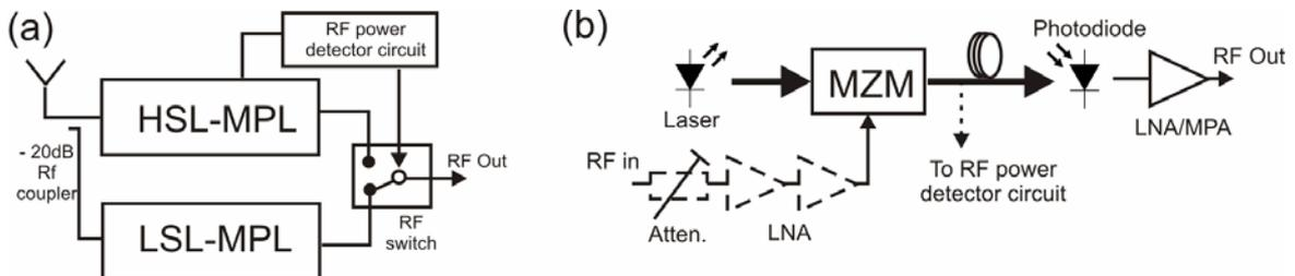
Fig. 1: (a) Schematic showing the EDR-MPL with dual link architecture and (b) Simulation model used to analyse both the HSL and LSL.
