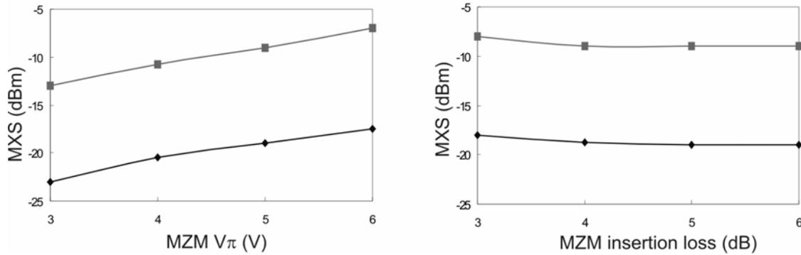
Fig. 6: MXS for the LSL against (a) MZM half wave switching voltage and (b) MZM insertion loss. The diamonds represent LSL with a pre-amplifier and squares represent LSL with an additional 10 dB attenuator.
