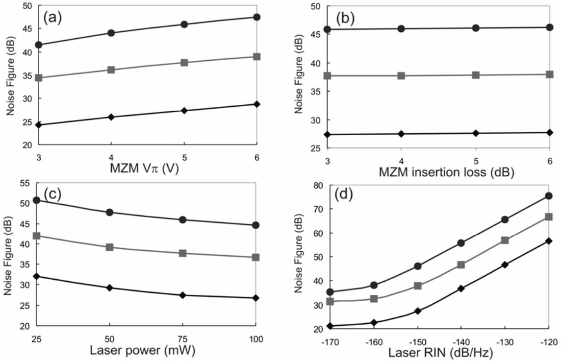
Fig. 5: Noise Figure for the LSL against (a) MZM half wave switching voltage (b) MZM insertion loss (c) laser power and (d) laser RIN. The diamonds represent LSL with a pre-amplifier with 30 dB gain and squares with an additional 10 dB attenuator. Circles are with a -10 dB RF coupler without any amplifier or attenuator.
