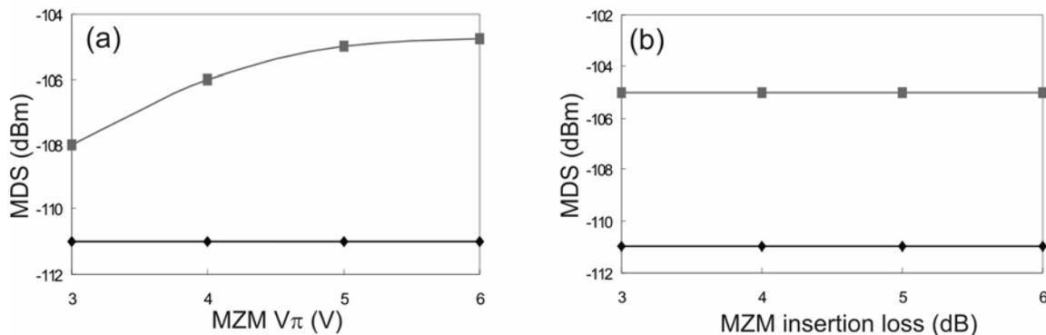
Fig. 4: MDS for the HSL against (a) MZM half wave switching voltage and (b) MZM insertion loss. The diamonds represent HSL with two cascaded pre-amplifiers with 30 dB gain each and squares are for HSL with one 35 dB pre-amplifier.
