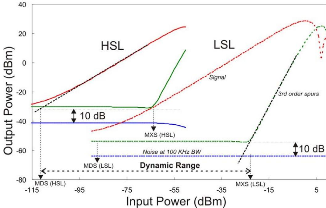
Fig. 2: Output power vs Input power for typical HSL (solid) and LSL (dashed). The figure also depicts the defined MDS and MXS parameters for both the HSL and LSL.
