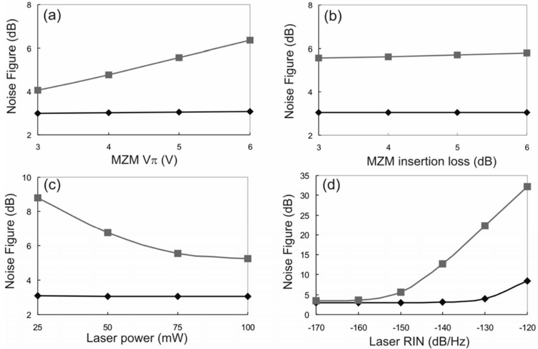
Fig. 3: Noise Figure for the HSL against (a) MZM half wave switching voltage (b) MZM insertion loss (c) Laser power and (d) Laser RIN. The diamonds represent HSL with two cascaded pre-amplifiers with 30 dB gain each and squares are for HSL with one 35 dB pre-amplifier.
